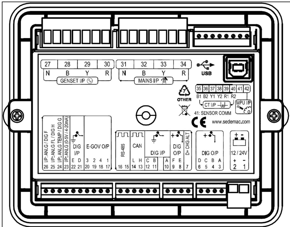
Figure 1: GC1031 Genset controller from the backside
